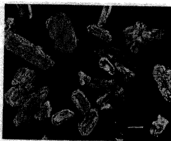
FIG. 8. Photomicrograph of bassanite from run 132. Starting material: gypsum and halite. 19 days at 70° C, with excess solid. Solution composition at end of run: 6.4 g \text{CaSO}_4 ; 374 g NaCl, per kg \text{H}_2\text{O} . Crossed nicols. The bar represents 0.1 mm.
